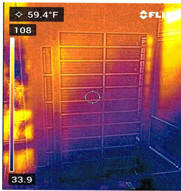
Figure 12. Thermal image of side of VRV condenser. Note warmer temperature on upper left of condenser and cooler to bottom right.
