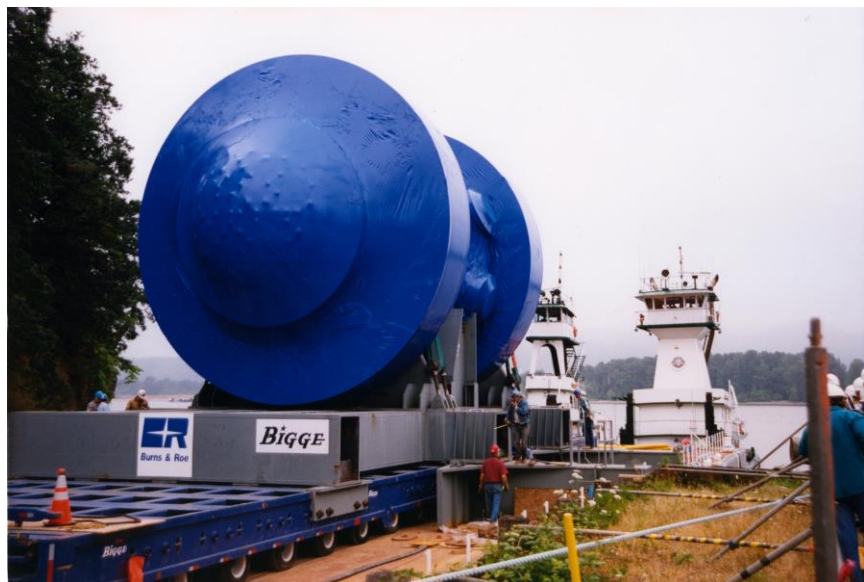
In 1999, PGE transported the Trojan reactor vessel and its internal components to the Hanford Nuclear Reservation disposal facility. The 1,020-ton package was safely transported by a specially made barge pushed by two tugboats 270 miles up the Columbia River.
