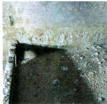
Midships Forward Bulkhead Pitting
