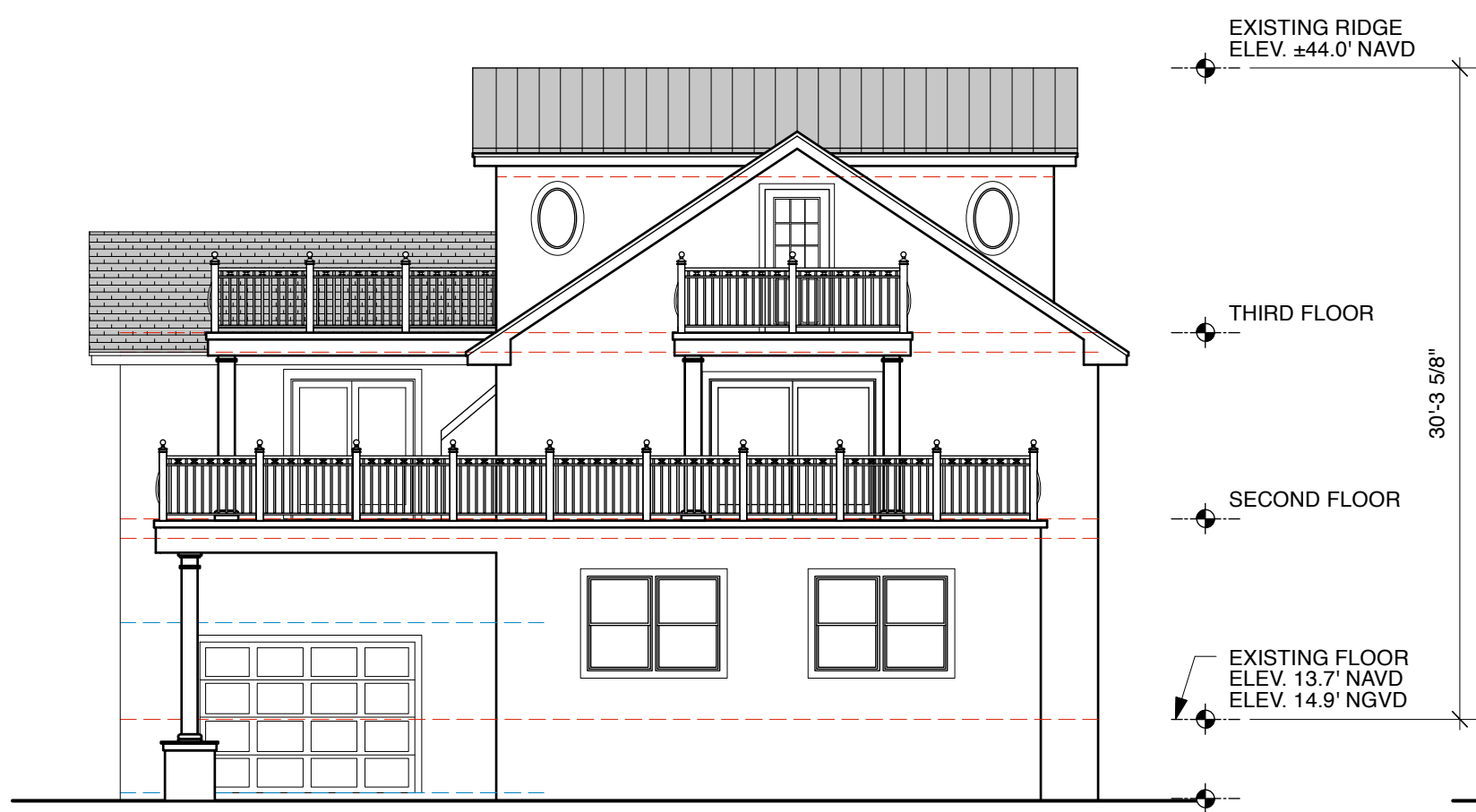
1 EXISTING FRONT ELEVATION 1/8" = 1'-0"
