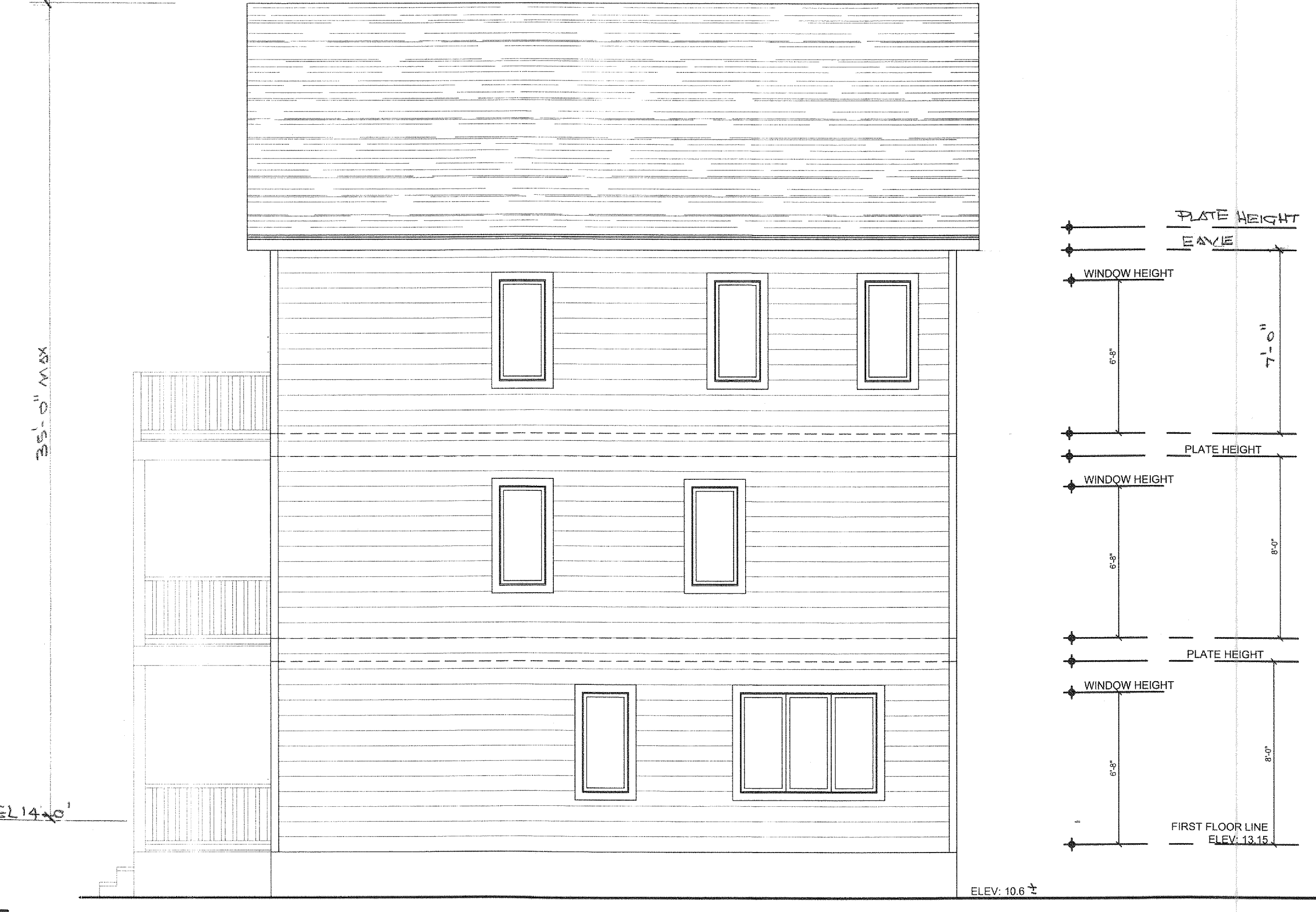
RIGHT SIDE ELEVATION PLAN 1/4"=1'-0"
