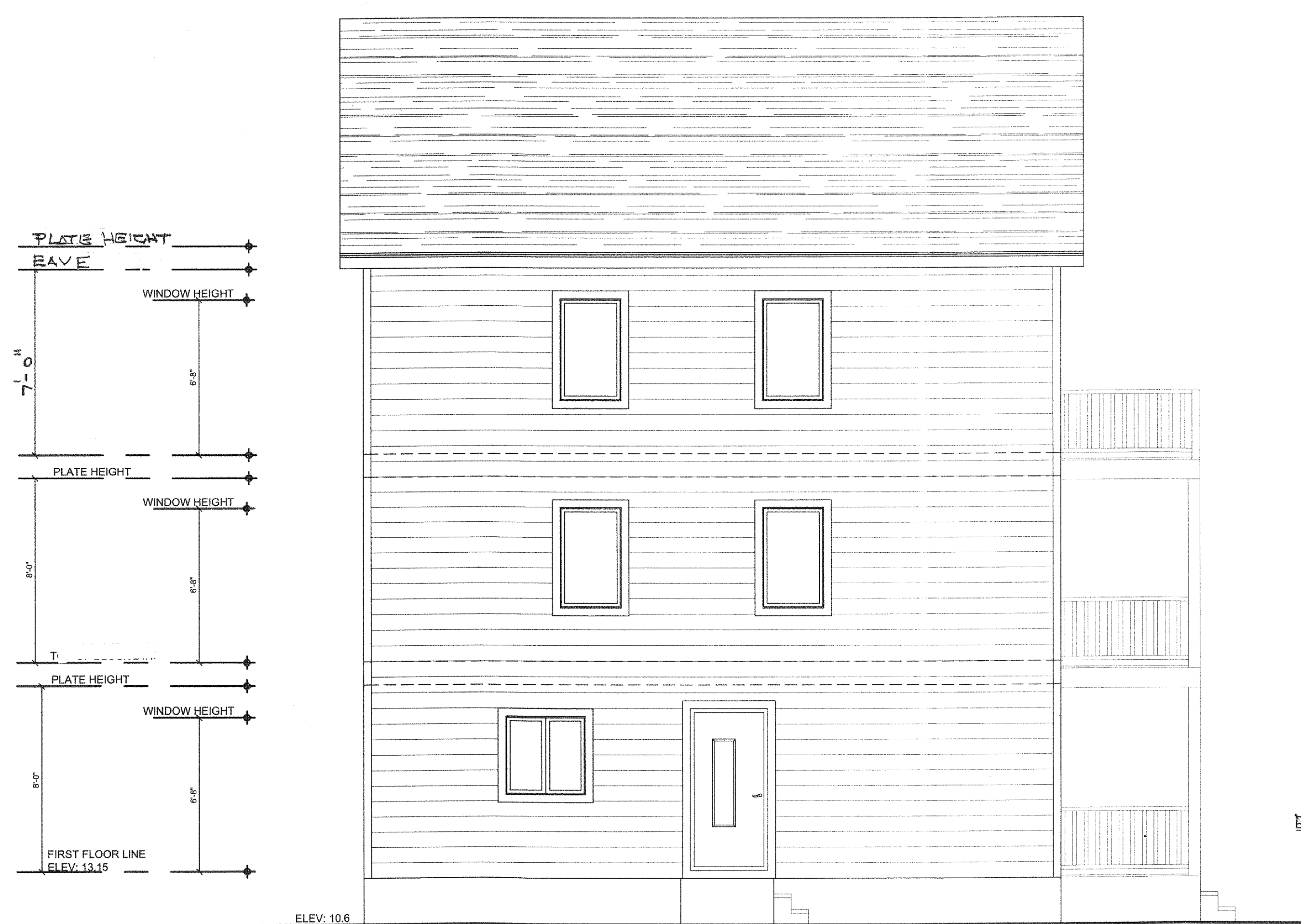
LEFT SIDE ELEVATION PLAN 1/4"=1'-0"
