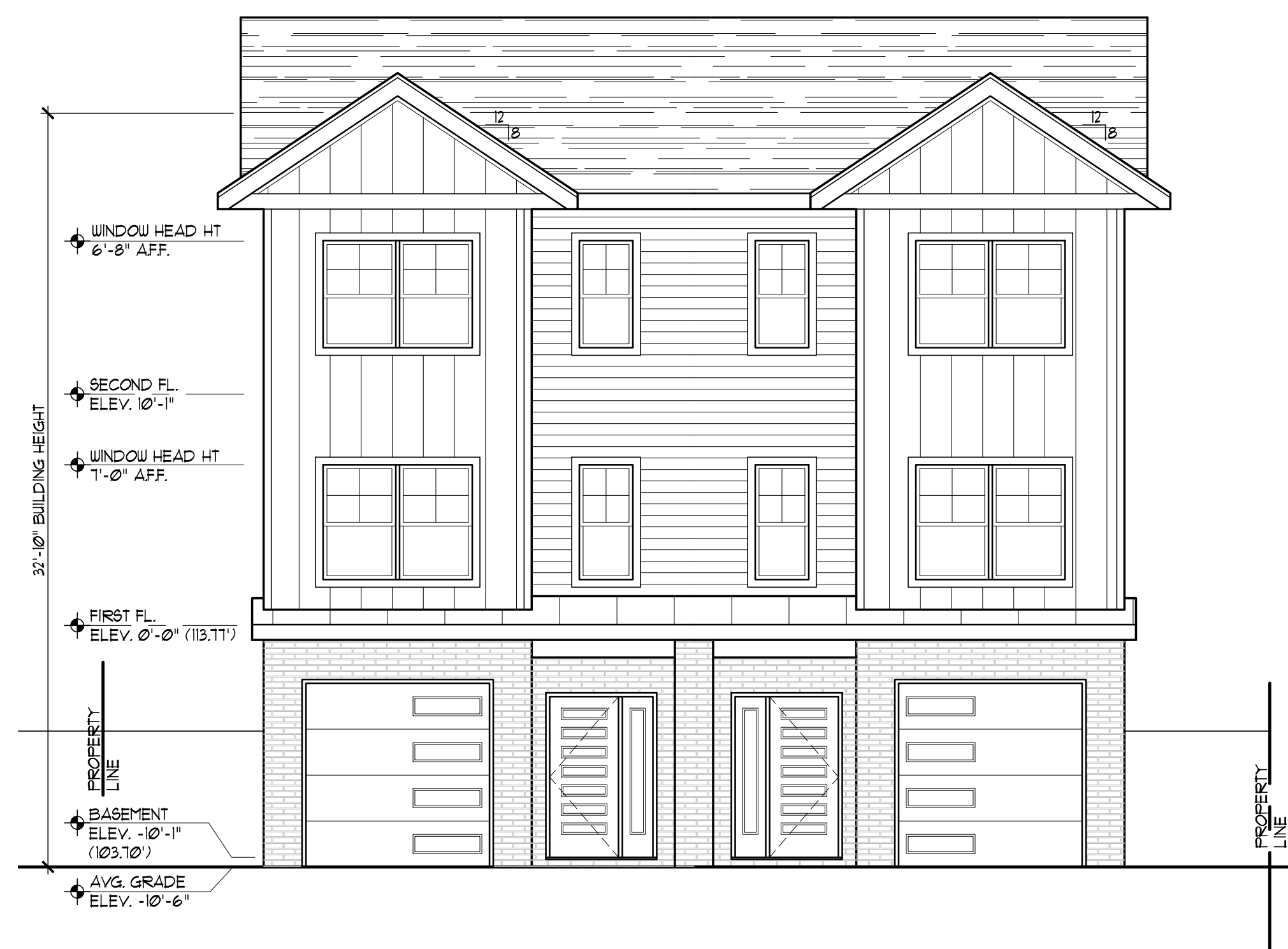
PROPOSED EAST ELEVATION SCALE: 3/16" = 1'-0"
