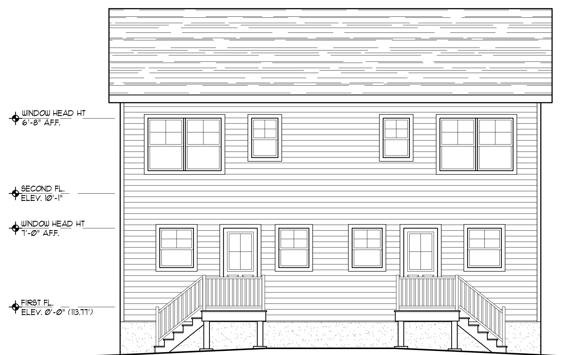
PROPOSED WEST ELEVATION SCALE: 3/16" = 1'-0"
