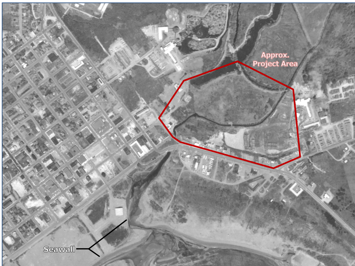
Figure 2-5. Crop from 1965 aerial photograph. Seawalls constricted the estuary downstream of the highway while sawmilling expanded north of the Project Area.
