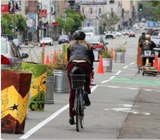
Example of a pop-up bike lane using pavement tape to designate the lane, and planter boxes/public art as buffers between the bike lane and vehicle travel lanes. (Source: AARP Livable Communities, "Project: Pop-Up Protected Bike Lane")
