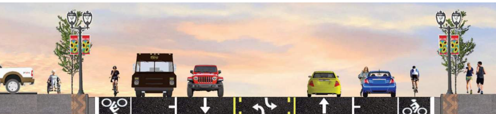
Figure 20: Bike lane with physical buffer (parking lane)
