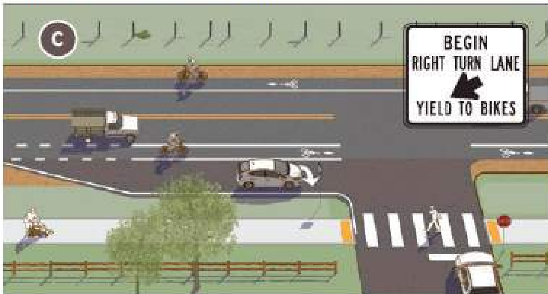
Figure 24: A variety of design treatments exist depending on the roadway configuration, available curb-to-curb width, traffic volumes and desire to provide a dedicated turn lane. All designs should strive to reduce speeds of turning vehicles, remind users of bicycle priority, and clarify user positioning approaching and through the intersection. Common signs at intersections include R4-4 "Begin Right Turn Lane Yield to Bikes" and a modified R10-15 "Turning Vehicles Yield to Bikes" sign.
