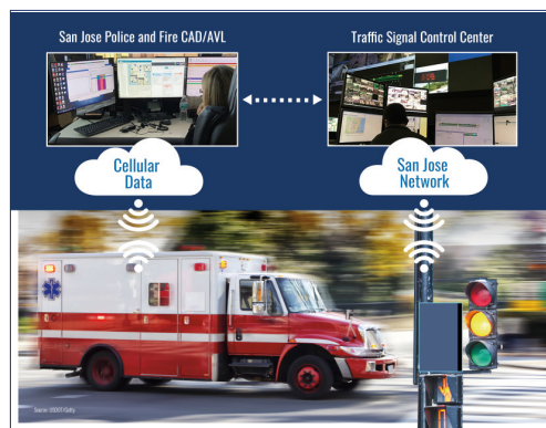
Figure 3. Illustration. System-based arrangement of emergency vehicle preemption. (Photo Credits: Enforcement Engineering, Inc. and Getty Images.)
